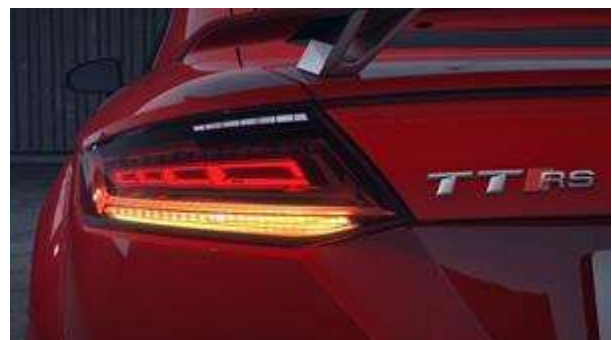
OLSA's unique OLED tail lamp on the Audi TT.
