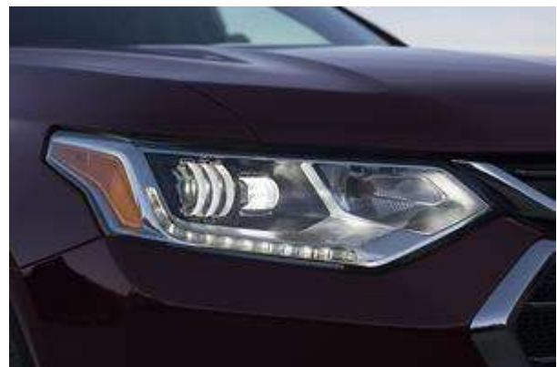
Magna's industry-first D-Optic LED headlamp on the Chevrolet Traverse.
